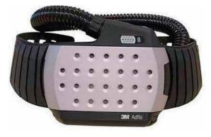
The airflow is always a constant nominal rate of 170 litres per minute, regardless of the battery's charge or the particle loading of the filter. For hot, humid jobs, you can increase the airflow to 200 litres per minute by simply pushing the ON button a second time
