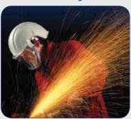
The individual respirator systems can be used in a variety of workplace applications. They include powered air respirators with integrated head, eye, face and respiratory protection and supplied air regulators with half and full face masks.
